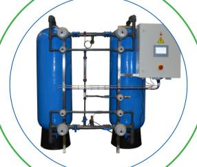
Filter media: a support layer (1,7 - 2,5 mm) protects the distribution system and improves the water distribution over the full surface of the vessel. The mono cation exchange resin is food grade certified, has a high capacity and a good physical, chemical and thermal stability. A top layer of inert resins finishes the packed bed and allows efficient water distribution.
